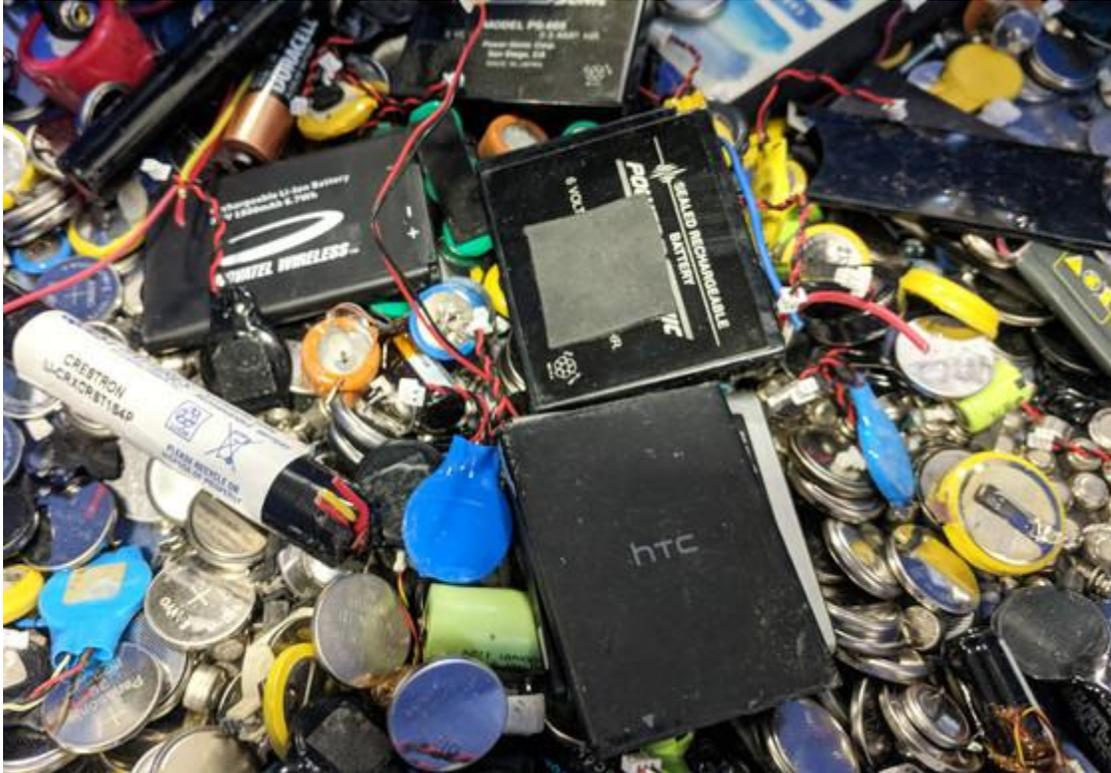
*Many batteries, especially powerful lithium-ion batteries in small electronics, can spark or react in ways that can lead to a fire. / Photo Credit: Neil Peters-Michaud/Cascade Asset Management*
